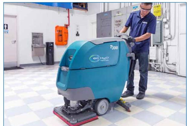
**5** Operate at a slow pace to effectively remove the most amount of floor finish. Scrub the area and repeat as needed to remove any additional floor finish.
